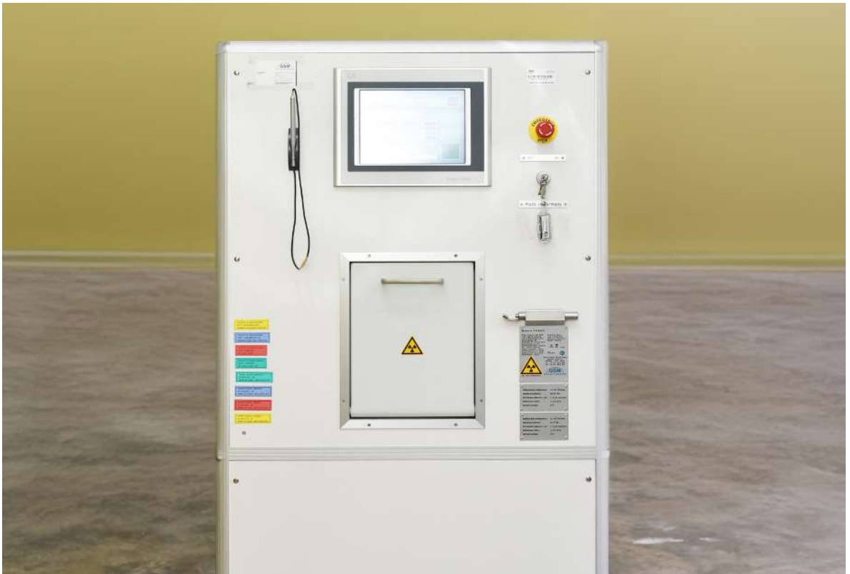
Self-contained gamma cell irradiator, Biobeam GM 8000 (Gamma Service Medical GmbH, Germany)
