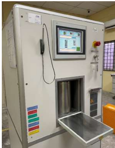
Figure 10. Self-contained gamma cell irradiator, Biobeam GM 8000 (Gamma Service Medical GmbH, Germany)
